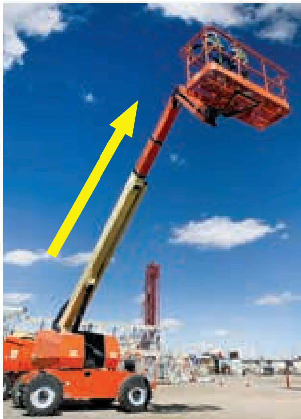
Figure 4-2 Telescope the Boom
