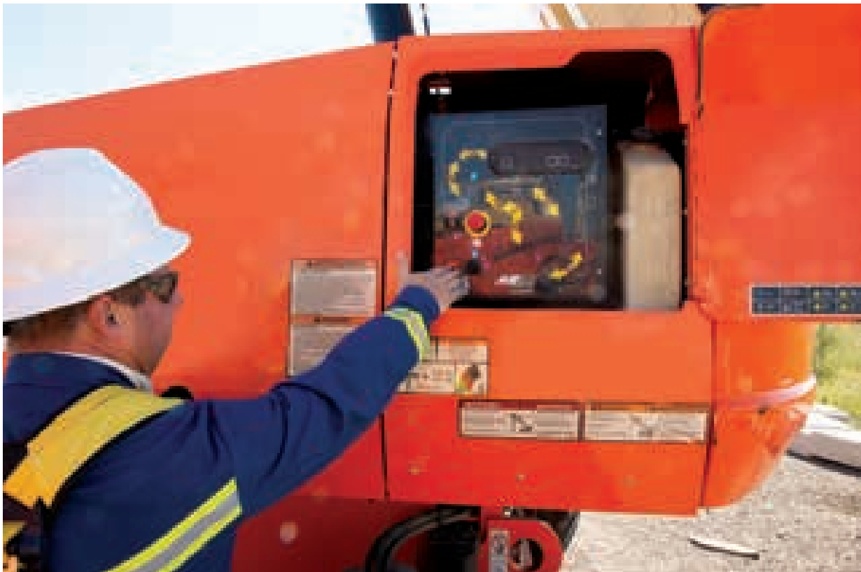
Figure 3-2 Ground Controls Function Test
