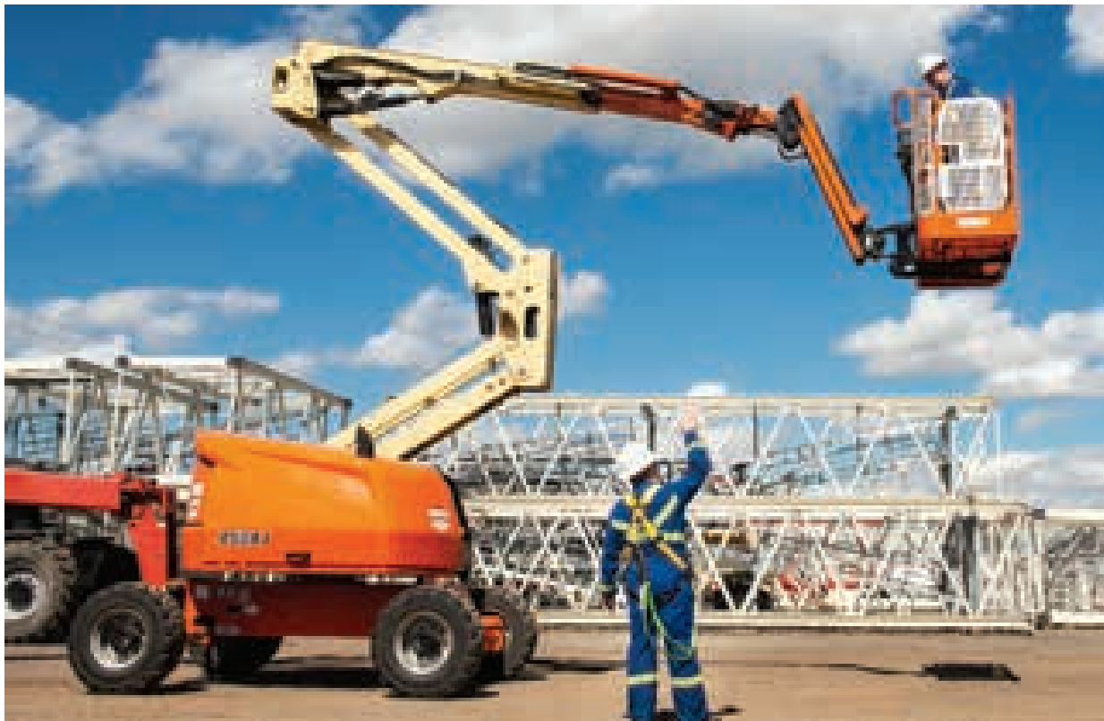
Figure 1-4 Spotter Monitoring a MEWP Operator
