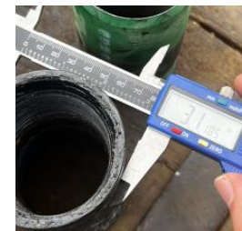
Pup joint with a regular collar (3.1").
