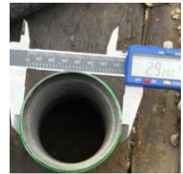
Pup joint with a Slimhole collar (2.9").
