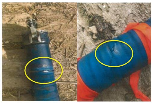
FAILURE IN TWO SECTIONS OF THE HOSE CONTRIBUTED TO INVERT RELEASE
