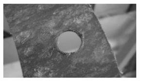
Example of asbestos gasket
