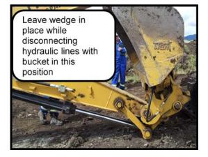
Once hydraulic lines are disconnected, place bucket in this position, to remove the wedge.
