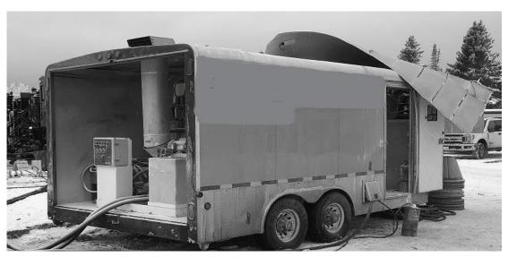
The flash fire blew out the back doors and the roof of the mobile heater unit, and caused damage to internal equipment
