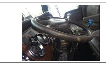
Damage to steering wheel from the impact of the driver's chest hitting it.
