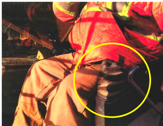
Operator jacket engages control stick (re-enactment)
