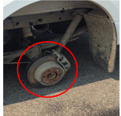
BROKEN AND MISSING LUG NUTS AND BOLTS
