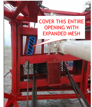
View of engineering guard to prevent improper spooling of drill line
