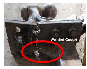
THE HITCH WAS RELOCATED TO THE UPPER MOUNTING POSITION AS EMERGENCY MEASURE TO REMOVE THE COMPRESSOR FROM THE HIGHWAY.
