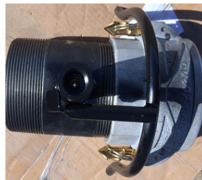
Examples of safety devices which reduce risk of fluid spilling or spraying; devices do not allow decoupling while there is pressure in the line
