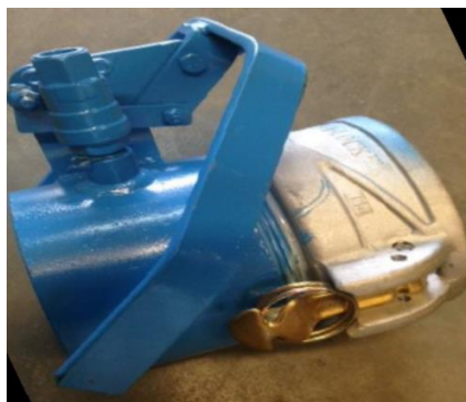
Examples of safety devices which reduce risk of fluid spilling or spraying; devices do not allow decoupling while there is pressure in the line
