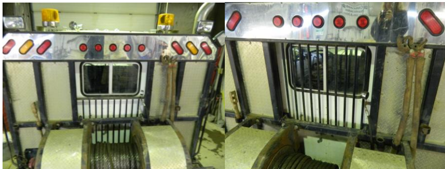
Window guard was not secured during task
