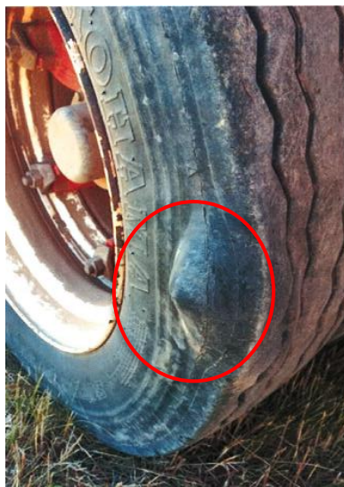
The electricity from the overhead line went through the truck and exited the sidewall of the steel-belted tire
