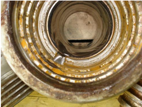
Figure 29. Washed Out Swivel
