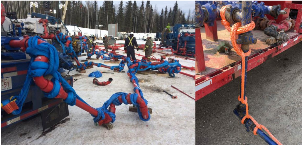
Figure 39. In-Series, Half Hitch Restraint System
