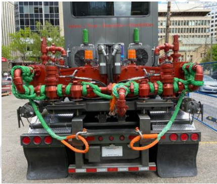
Figure 32. High Pressure Piping on Twin Pumper with Restraints
