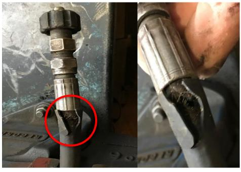
The steam hose ruptured just below the crimped fitting
