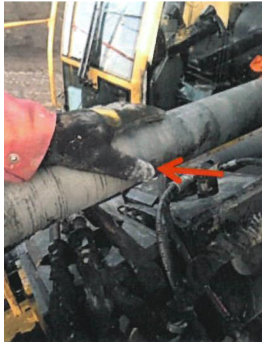
Arrows indicate direction of jetted hydraulic fluid from the fitting to the left thumb (re-enactment)
