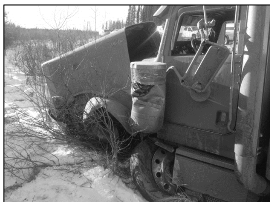
Damaged truck cab located in ditch
