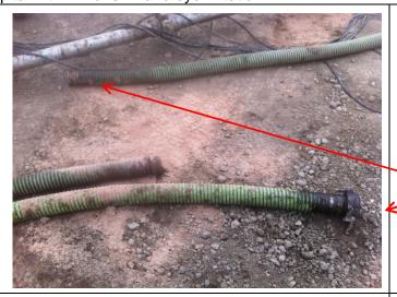
Hoses with two male ends being held together by hand during incident
