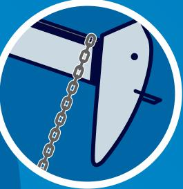
CHAINS OVER THE BEAM Engineered chain loop? Chain and boomer appropriate for load?
