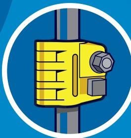
POLISHED ROD CLAMP Proper clamp for load? Proper bolt torquing?
