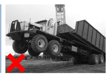
Unacceptable risk resulting from shale bins being loaded when overweight
