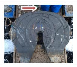
Fifth wheel pin/washer out of locking position
