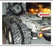
Snow and ice not cleaned properly before trailer coupling
