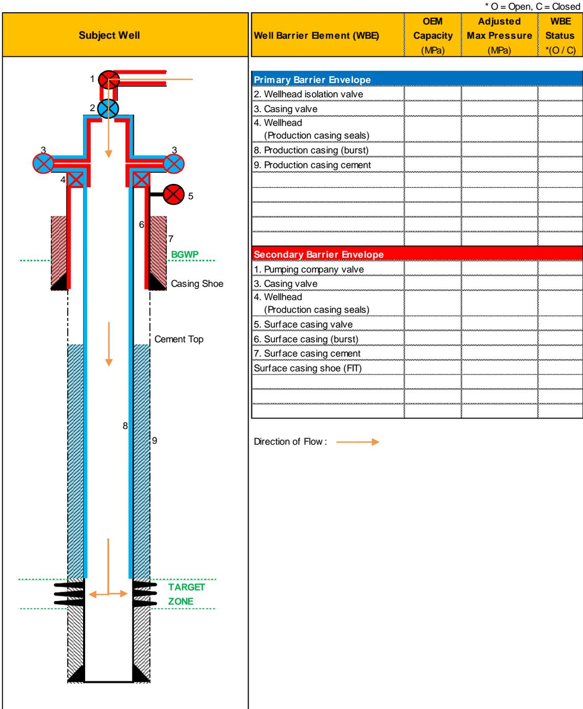
**Sample Subject Well fracture string completion schematic.**
