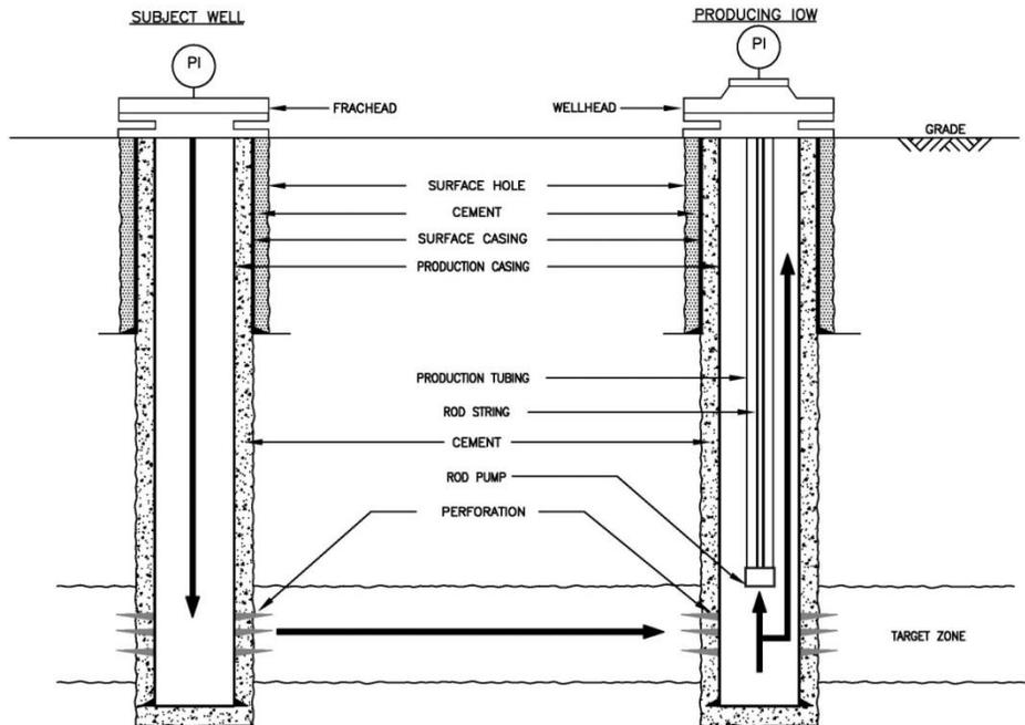
**Step 2. Based on the flow path scenarios, identify primary and secondary barrier envelopes within each at-risk IOW. These may be illustrated on a barrier schematic. (See [Appendix D](#) for a sample barrier schematic and the Hazard Register for a blank barrier schematic template.)**
