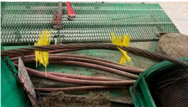
Example of sand line flags installed before use
