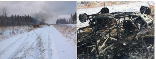
UTV ROLLED OVER INTO DITCH AND THE SPILLED FUEL IGNITED DESTROYING THE VEHICLE
