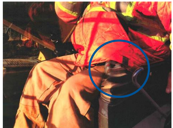
Jacket caught on boom controls. (image source: Energy Safety Canada Safety Alert 02-2016 )
