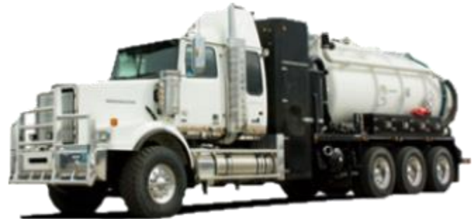
Typical combo vac unit.
