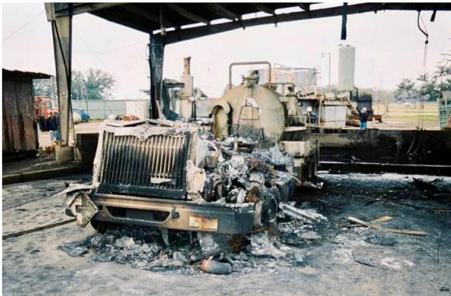
**Destroyed vacuum truck following an engine runaway fire and explosion**
