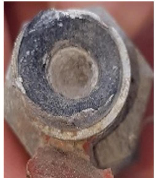
PRESSURE RELIEF VALVE HAD A BUILDUP OF SCALE
