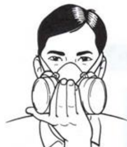
Figure 2: Positive Pressure Seal Test
